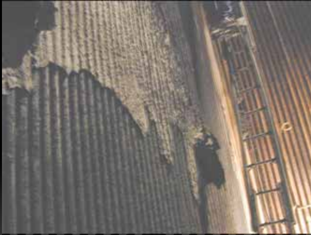
Oxistop Coating Shedding Slag
